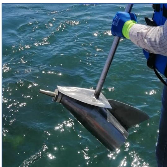
Figure 2. depth-integrating suspended sediment sampler
